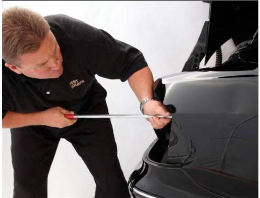
**Working on a rear fender dent through the taillight opening.**
