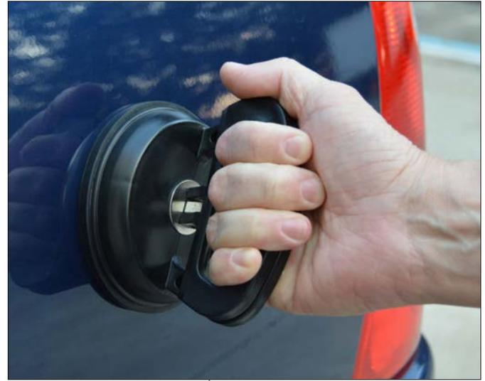
**A suction cup puller being used for dent removal.** (Image: AAA)
